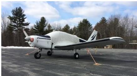
All aircrafts stored outside must be located on an approved airport tie down spot and the aircrafts are required to be chocked and tied down using the standard three point tie down system. All aircrafts stored in either Terminal Hangar A, Terminal Hangar B, or Tiedown area on the Apron, are subject to the fees associated with those locations.
